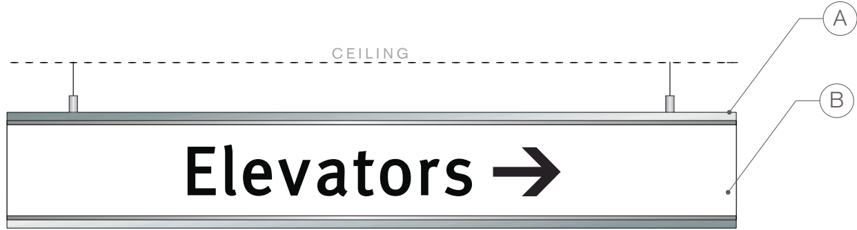
Type C.2-1S V711-3S 44.0"w X 7.0"h Double Sided Overhead, Accommodates 5.82"h Insert
