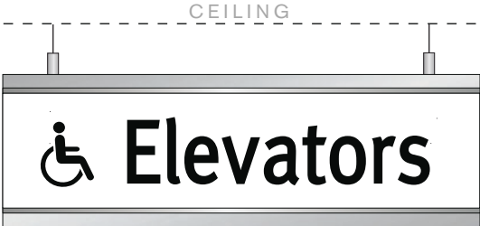
Type C-1S V511-3S 22.0"w X 7.0"h Double Sided Overhead, Accommodates 5.82"h Insert
