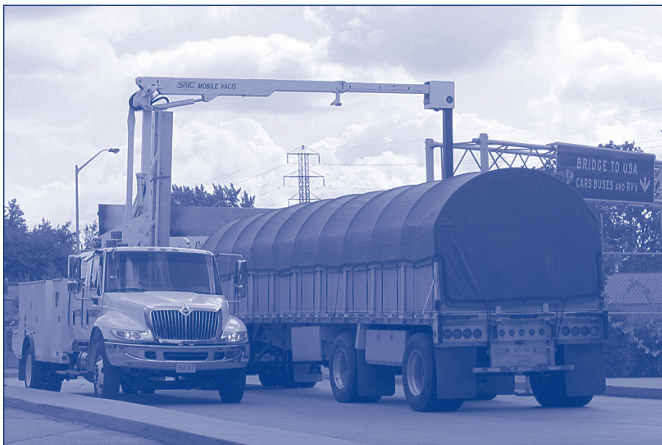
Inspecting cargo via gamma ray imaging at the Detroit-Windsor gateway, the nation's and the world's busiest border.
