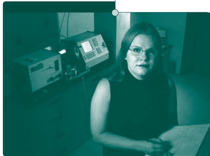
Dr. Stephania Messersmith with an atomic absorption spectrometer, an instrument used by forensic scientists to analyze samples for gunshot residues or revealing soil or toxicological matter.
