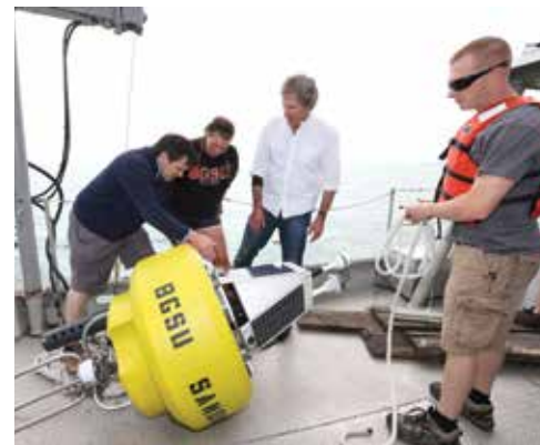
It's a buoy! And it's one of BGSU's high-tech sensors placed in Sandusky Bay and Lake Erie that report on pigments, pH and other variables. "These sensors can tell you what's happening in real time and they can make adjustments on the fly," said Bullerjahn, pictured with Mike McKay and two students. The data is uploaded by satellite directly to the team's cellphones.
