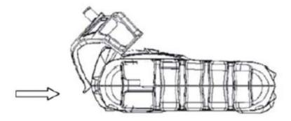
· Press both side tabs down onto instrument until they snap in.
